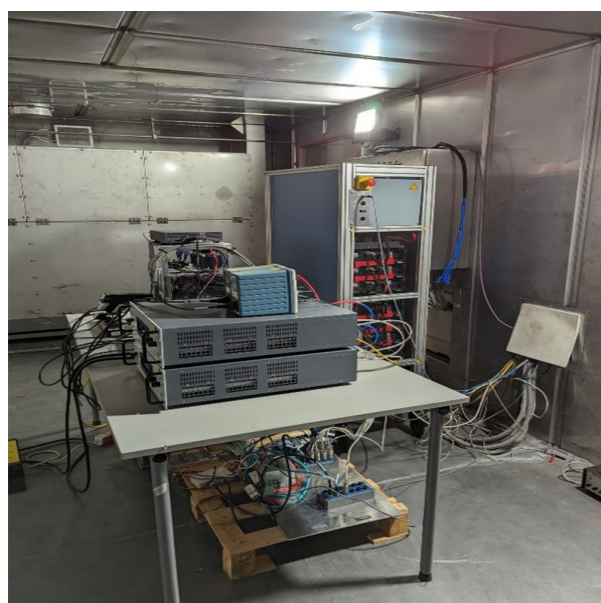
Fig. 9 Test setup of battery EIS
