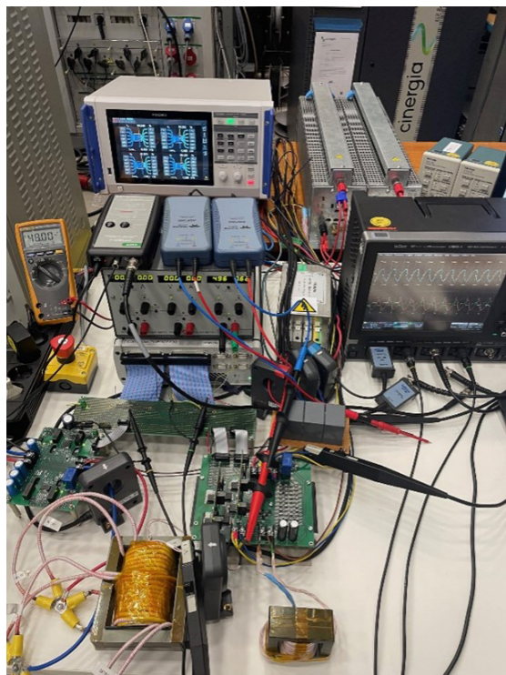
Fig. 8 Test setup of series resonant AC/DC converter
