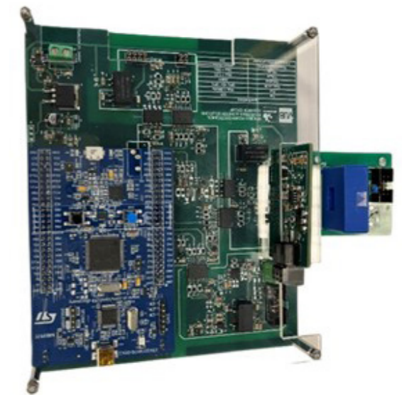
Fig. 6 PHM circuit of DSC-based DAB converter
